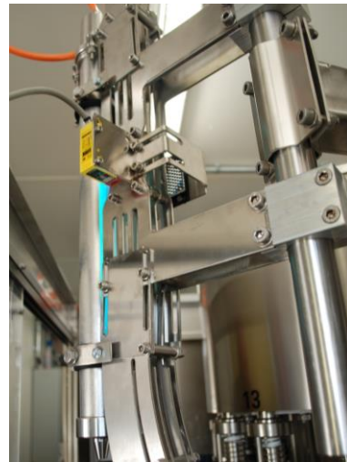
steriBELT module in front of trailing caps right before cap sealing system
