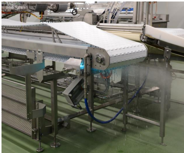
steriBELT module during spray water cleaning process (CIP)
